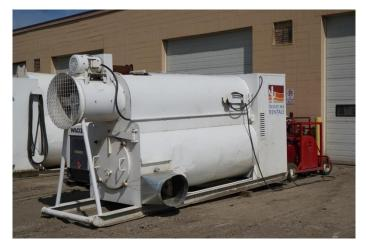
Unit Name: DAR005 Type: Lister Capacity: 2.5 million BTUs (2.6 million kJ) Skid mounted Uses No. 2 (diesel) fuel
